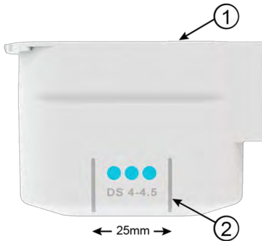
Figure 3.4: Image/Treat transducer separated from handpiece (see Table 3.3)
