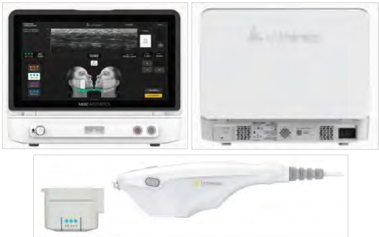
Figure 3.1: Main components of the Ulthera® System: control unit (top), handpiece (bottom right), and image/treat transducer (bottom left) that inserts into the handpiece receptacle.
