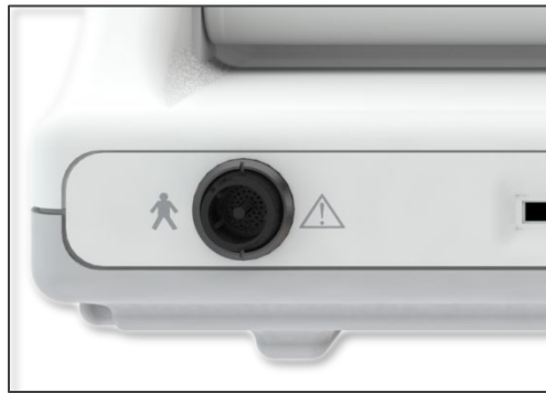
Figure 5.1 Handpiece Connector Receptacle.
